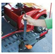
Self-tensioning retractable securement belts.
