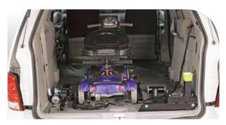
Take-apart lift disassembles when not in use if desired.
